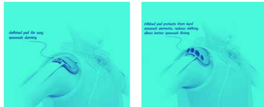
One of the early proposals of the Airbag Protection System – Deflated and Inflated
